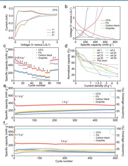
Figure 3. Electrochemical characteristics of the various anodes in half cells. (a) First three CV curves; (b) first discharge/charge curves at 0.05 A  $g^{-1}$ ; (c) rate capabilities at different current densities from 0.05 to 5 A  $g^{-1}$ ; (d) comparison of capacities between this work and other literature; (e) cycling stability of the four electrodes at 1 A  $g^{-1}$  and (f) 5 A  $g^{-1}$ .
