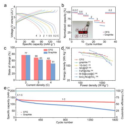
Figure 5. Electrochemical performance of the CFG//LFP full cells ( $1C = 150 \text{ mAh g}^{-1}$ , based on active material in cathode). (a) Charge/discharge profiles of LFP//CFG full cells at different currents; (b) rate performance between 0.2 and 4 C; (c) plot of SOC of CFG and graphite at each current density; (d) Ragone plot; (e) cycling performance of the CFG//LFP full cells at 1C.
