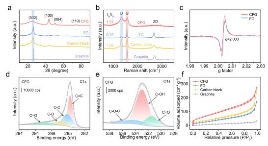
Figure 2. Physical—chemical properties of the as-obtained samples. (a) XRD patterns; (b) Raman spectra; (c) ESR spectra; (d) high-resolution XPS analysis of C 1s and (e) O 1s for CFG; (f) nitrogen adsorption/desorption isotherms.
