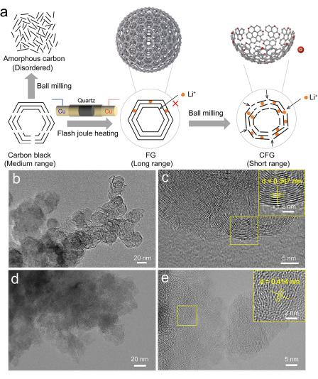
Figure 1. (a) Schematic illustration of the morphological structure of the conversion from CB to CFG. (b) TEM image and (c) HRTEM image of FG. (d) TEM image and (e) HRTEM image of CFG.
