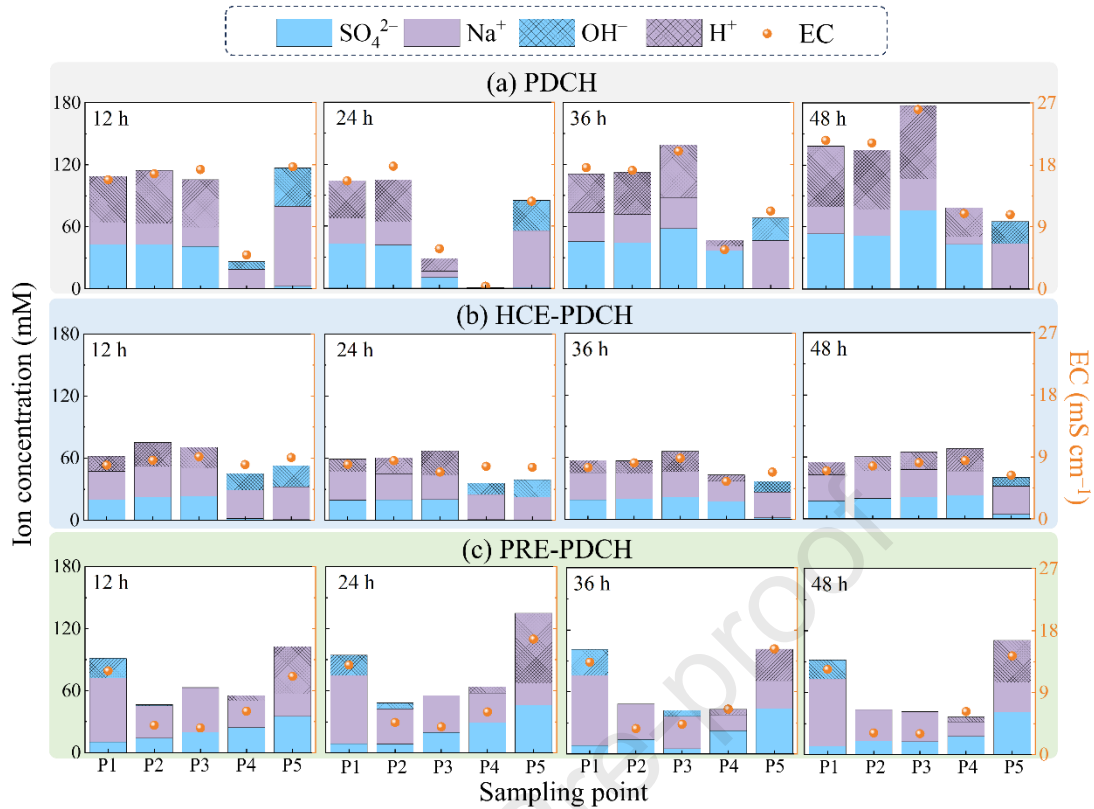
Fig. 4 EC and main ion concentration ( \text{Na}^+ , \text{H}^+ , \text{SO}_4^{2-} and \text{OH}^- ) distribution along the
