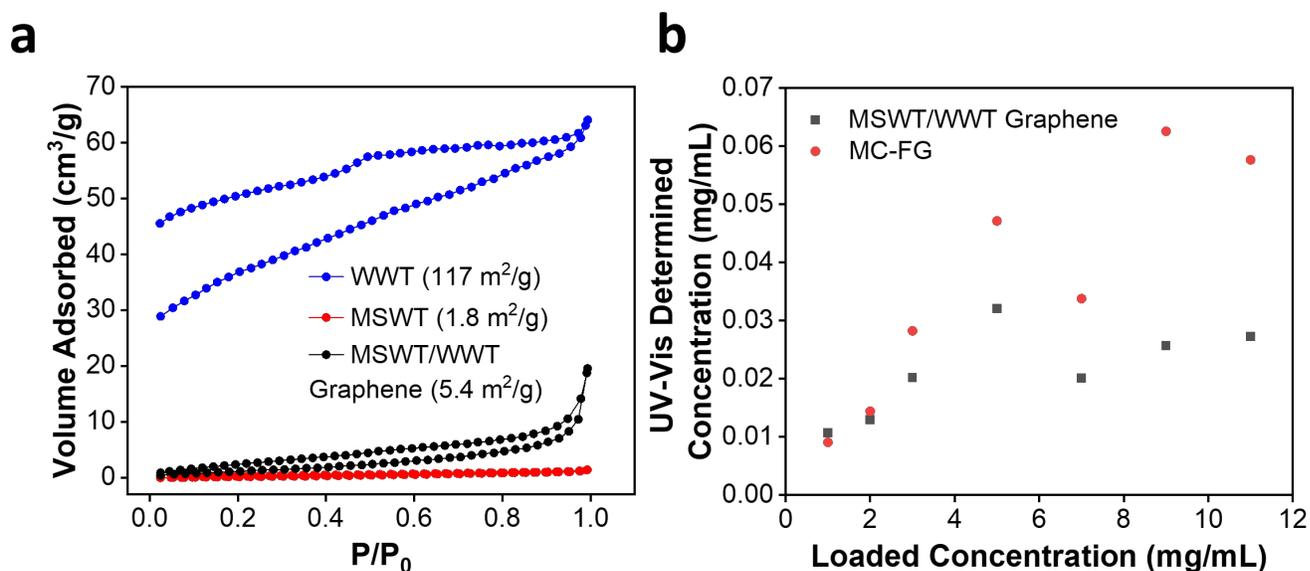
**Figure 5. BET analysis and dispersion in 1% pluronic F-127 solution of MSWT/WWT-derived graphene and MC-FG. a. BET analysis of feedstocks and resulting graphene. b. Dispersion of MSWT/WWT graphene and MC-FG in pluronic F-127.**
