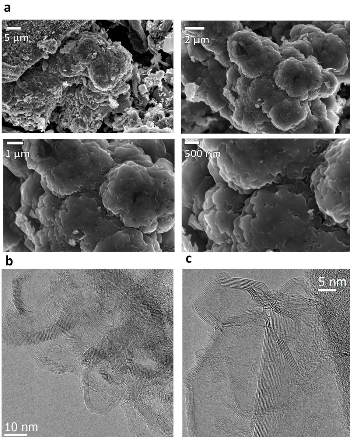
**Figure 4. Electron microscopy of MSWT/WWT graphene. a.** SEM images depicting sheet like morphology in MSWT/WWT graphene at various magnifications with associated scale bars. **b. and c.** TEM micrograph of MSWT/WWT graphene highlighting lattice fringes.
