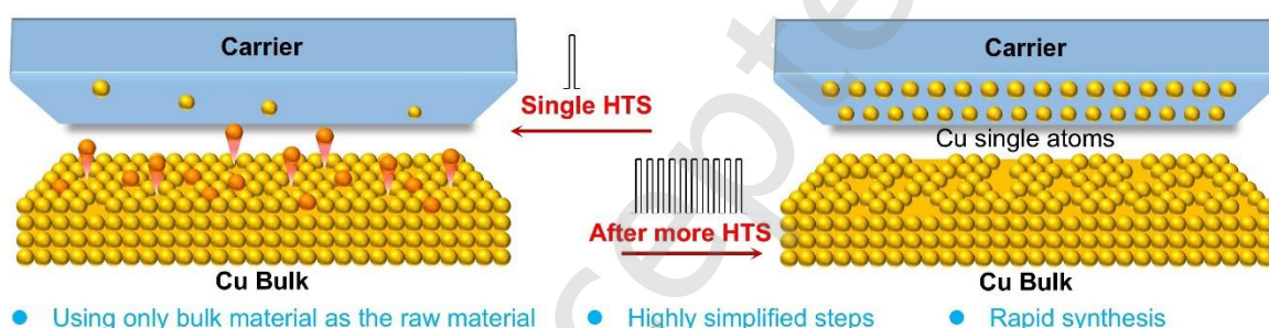
Figure 1. Comparison of different strategies for the synthesis of SACs. (a) Typical bottom-up strategies using wet chemical methods. (b) Typical thermochemical gas-assisted method for synthesizing Cu SAC. (c) Our proposed top-down strategy, where high-temperature shock (HTS) directly processes bulk copper to synthesize Cu SAC. (Blue, nitrogen atoms; white, hydrogen atoms; orange, iron atoms; yellow: copper atoms).
