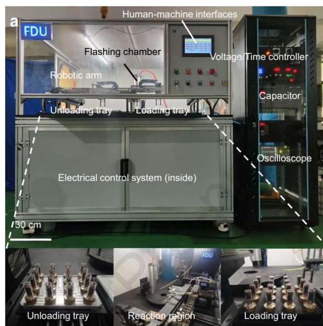
Fig 3. A photograph of a pilot-scale fabrication device of FG adapted from [26] under the creative commons license CC BY 4.0.
