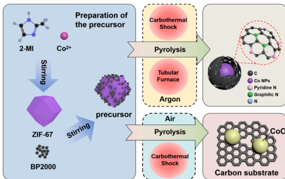
Fig. 1. Schematic preparation of Co@N/C-Joule, Co@N/C-Tube, and CoO/N/C-Joule catalysts synthesized by pyrolysis of ZIF-67.
