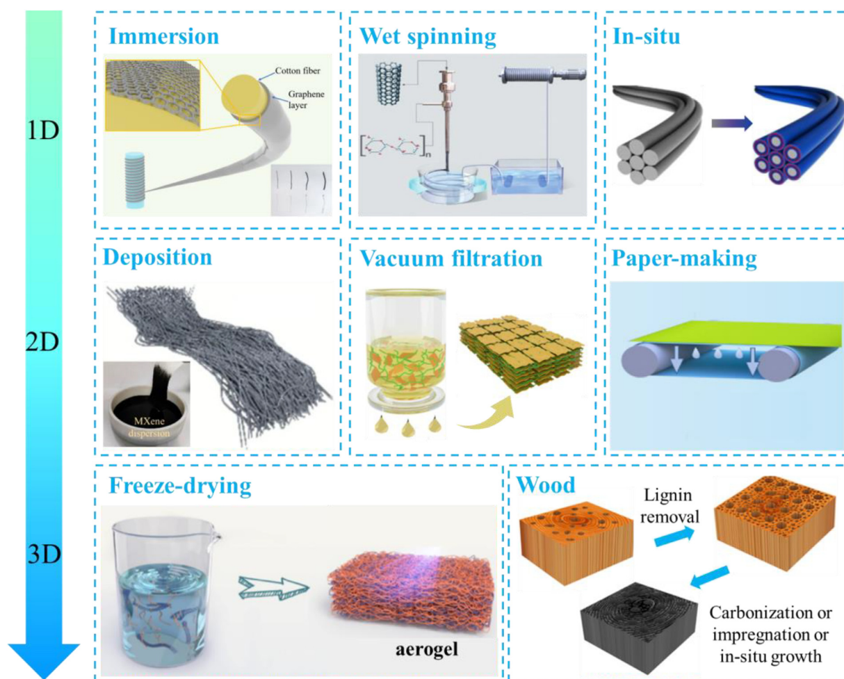
Fig. 2. Main preparation methods for 1D, 2D, and 3D cellulose-based Joule thermal devices. Immersion [56]. Wet spinning [57]. In-situ [68]. Deposition [97]. Vacuum filtration [101]. Paper-making [88]. Freeze-drying [133]. Wood [124].
